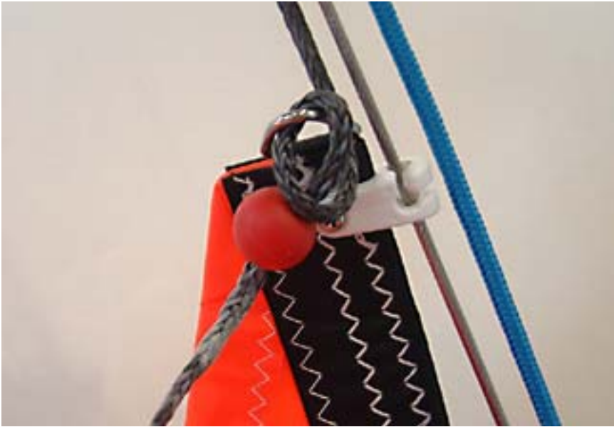
As with the main halyard, the jib halyard is slightly oversized. At left the attachment loose, below tight.
